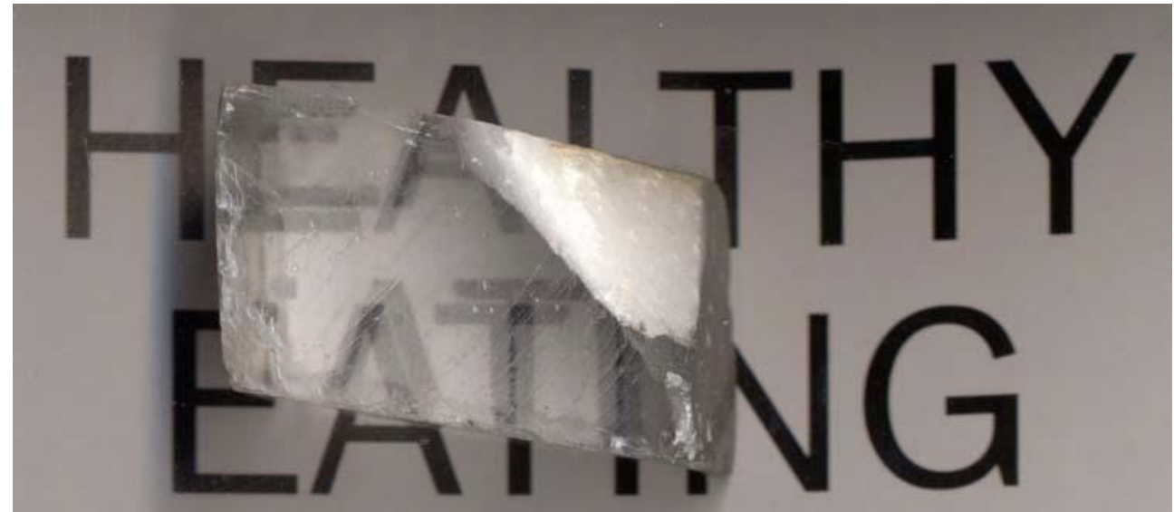
Birefringence in a calcite crystal
