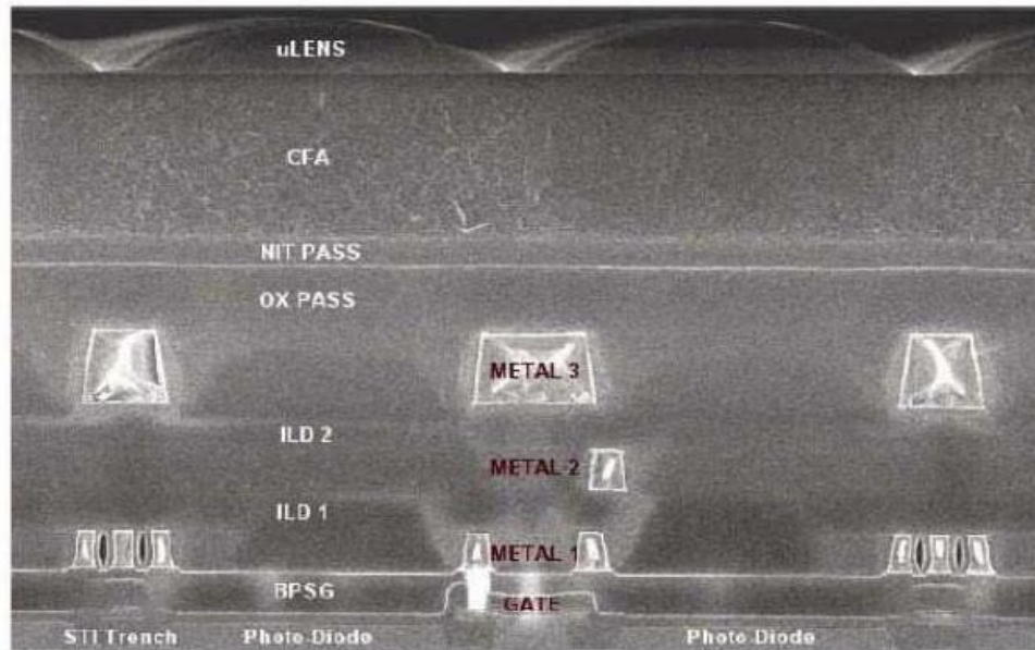
Sensor cross-section
