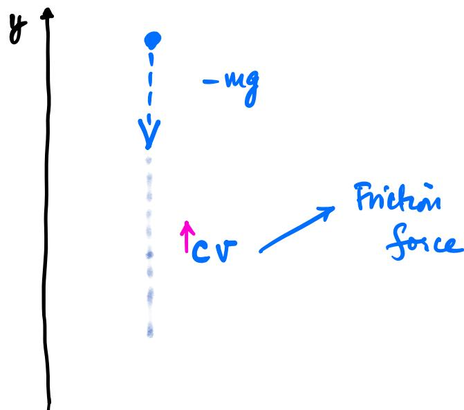
Force due to friction will continue to increase till it equates  $mg$ . At which point the ball will have no force acting.
