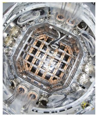
Image sensors that are chilled to -90 degrees Celsius by cryostate to eliminate noise.
